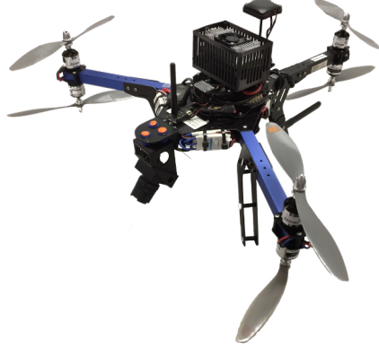
Figure 4.7: The 3DR Y6 multirotor used in hardware experiments. The Pixhawk autopilot runs APM:Copter firmware. The camera has a resolution of 800 \times 600 at 30 fps and is mounted at a 45-degree angle.
