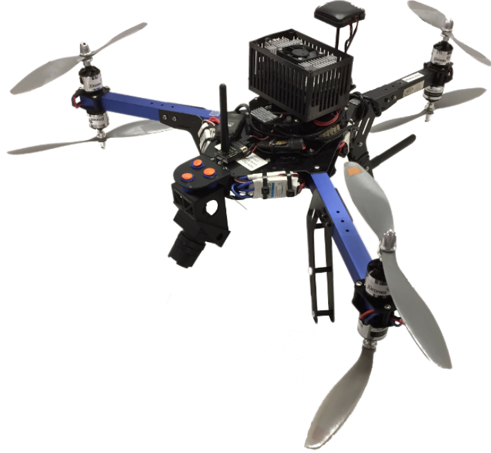
Figure 3.4: 3DR Y6 multirotor used in hardware demonstration. The Pixhawk autopilot runs APM:Copter firmware. The camera has a resolution of 800 \times 600 at 30fps and is mounted at a 45^\circ angle.
